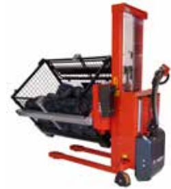
On the Rotator, lifting, lowering and rotation are controlled by cable remote control (as standard). Wireless remote control for lifting, lowering and rotation is available as optional extra.
